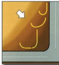
Figure 6. J-hook silt fences provide multiple storage areas
