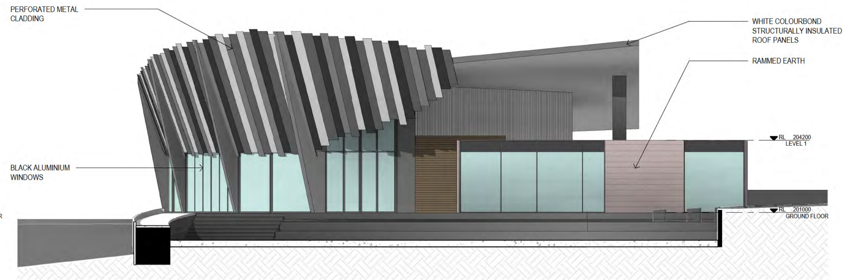
4 ELEVATION 1 : 100 SOUTH ELEVATION
